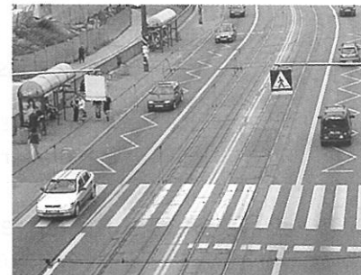
Zigzag lines on the road indicate that the motorist is approaching a pedestrian crossing.
